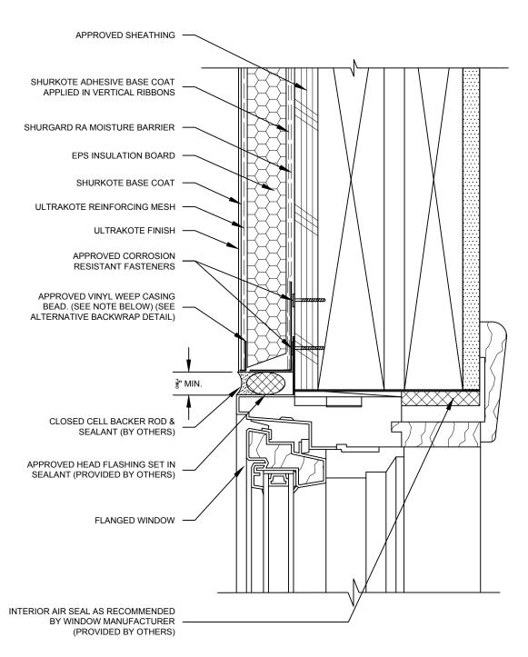
NOTE: MAINTAIN  $\frac{1}{8}$ " SPACE BETWEEN BEVELED INSULATION AND WEEP CASING BEAD.
